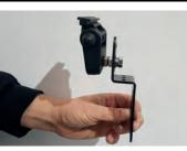
Fix each Centre Mount to the Bumper Beam brackets as shown using the supplied: bolt, 3x nuts, spring and penny washer (centrally on the middle mounting slot).
