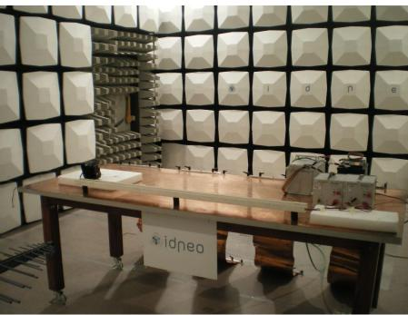
Figure 23. . RE Test. Test Setup from 200MHz to 1000MHz. WL80 G2
