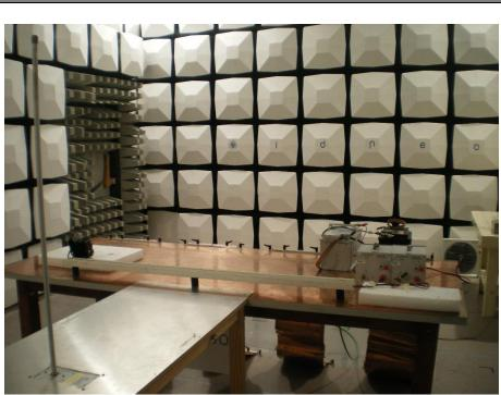
Figure 21. RE Test. Test Setup from 100kHz to 30MHz. WL80 G2
