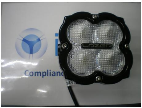
Figure 1. Sample under test WL45 G2 Lamp (Lens picture is not according to the production level).
