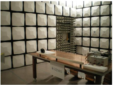
Figure 24. . RE Test. Test Setup from 1000MHz to 2500MHz. WL80 G2
