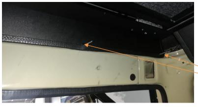
Once the holes have been drilled bigger, you can now proceed to fit the rear panel in place and insert the pop rivets
