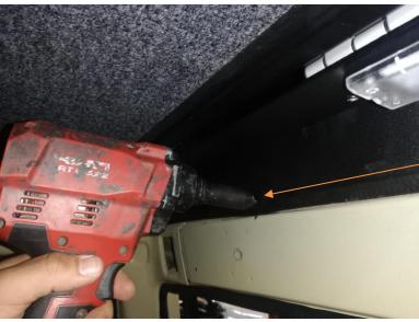
Use a pop rivet gun to secure the pop rivets in place.
