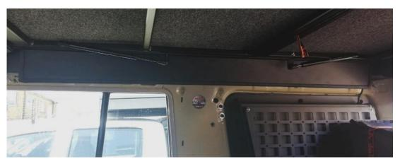
The rear panel should be fitted roughly into place and with a marker, the holes on the body that correspond with the cover plate should be marked out and drilled to 5mm in diameter.
