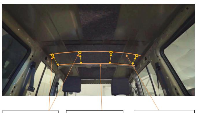
The distance from rear edge of the front top hat to the centre of the hole is 45 mm
