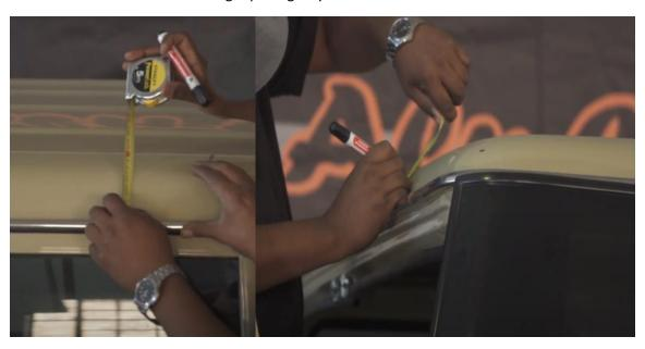
You will then need to drill access holes from the inside of the vehicle 45 mm from the rear edge of the front top hat using a 3 or 4 mm drill bit.
