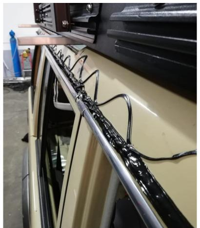
Apply Sika flex along the inside of the front face of the Thor roof conversion as well as the body of the vehicle above the windscreen.
