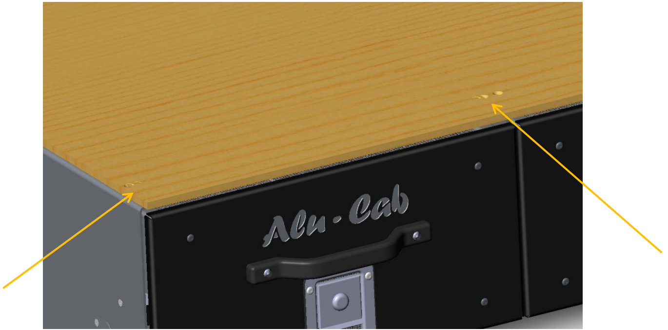
Figure 3: Once all the Bolts are removed you can remove the Drawer Top
