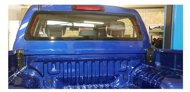
4. Images showing front mounting position of mounting brackets in load bin
