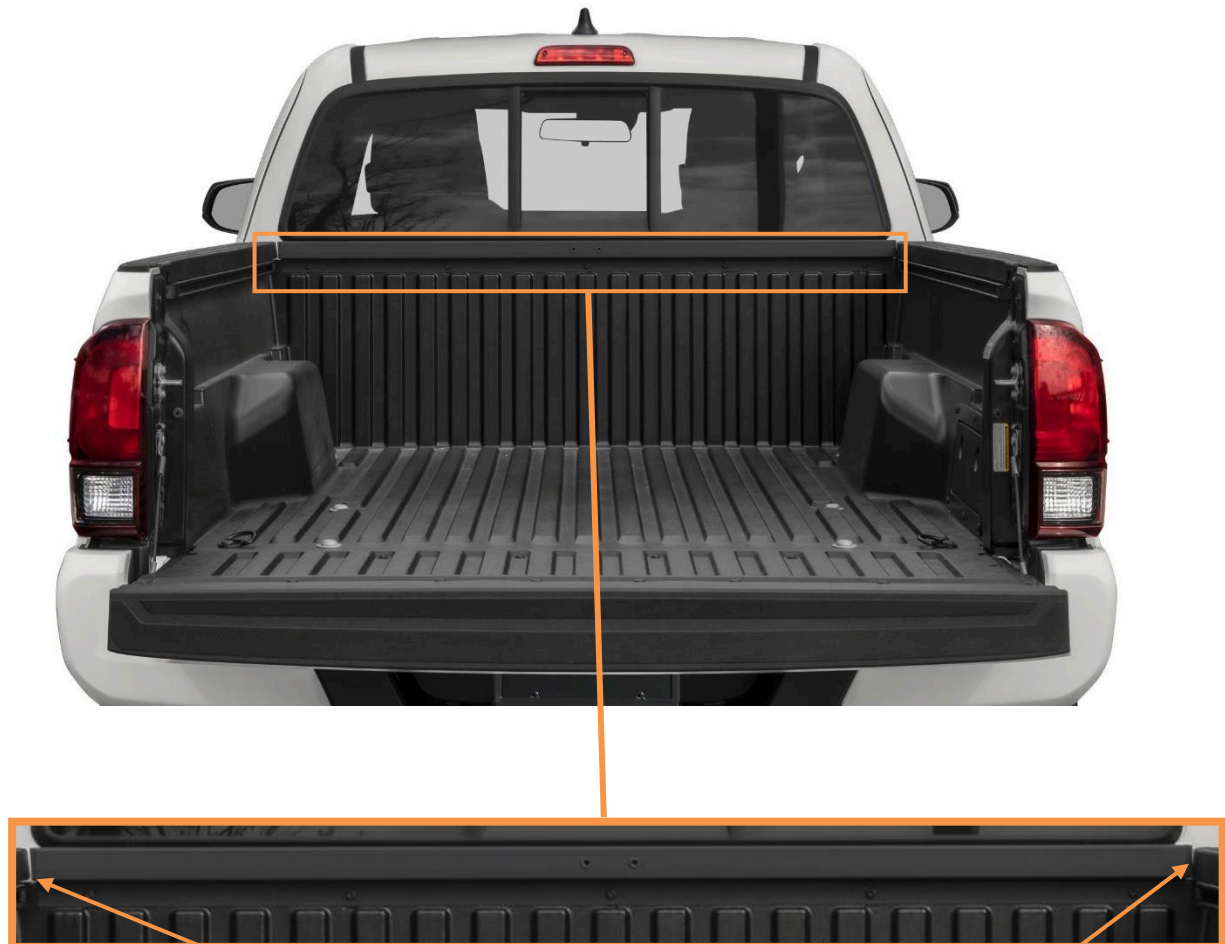
Fig 12: Gaps in Factory Bulkhead Spacer
