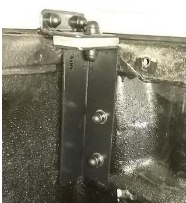
Figure 16: Front Support Bracket Installed
