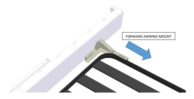
Test fit the front bracket supplied and mark the holes required to mount the awning. Drill through the awning with an 8mm drill bit
