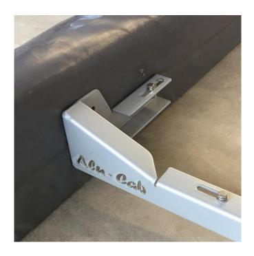
Pre-mount and fasten the front mount to the drilled holes.
