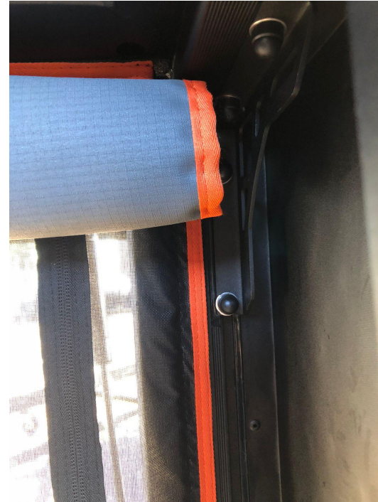
Figure 7: Side Door Mozzie / Midgie Net Installed
