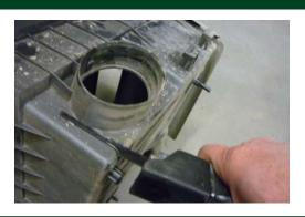
4. Using a die grinder, remove ribs from above hole as shown.
