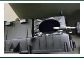
5. Using an air hacksaw, cut away lower side section of air box as shown.
