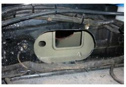
19. Temporarily place air box in position in engine bay. Through hole cut in mud guard, mark section to be cut away on inner panel. Remove air box.
