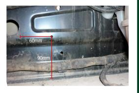
16. Using extreme care not to damage wiring loom, cut a hole using a 102mm hole saw as shown.
