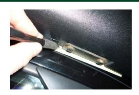
23. Hold pillar bracket in position previously marked and mark three mounting holes. Drill holes to 7.5mm.
