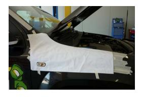
14. Drill six stud mounting holes to 16mm and 12mm as shown on template.
