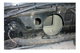
17. Mark second hole 90mm from top surface of wheel arch in engine bay and 70mm back from earth stud (if equipped) on inner guard (if not equipped refer to second photograph).
