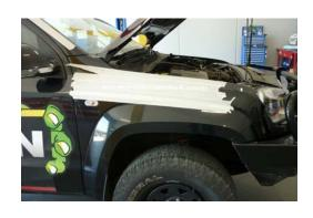
13. Tape template to mudguard making sure it is lined up with top of mudguard (bonnet opening) and rear of mudguard (door opening).
