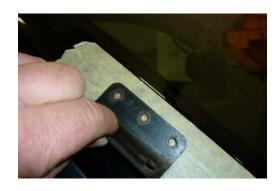
24. Apply silicone sealant. Insert mounting plugs and attach mounting bracket to screen pillar using self tapping screws provided.
