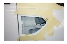
**5A.** Drill 2 x 16mm mounting holes using a step drill. De-burr and rust-proof exposed metal.
