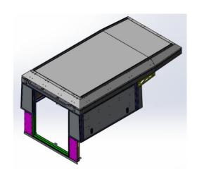
5.1. Connect rear filler panel assembly and base unit as shown.
