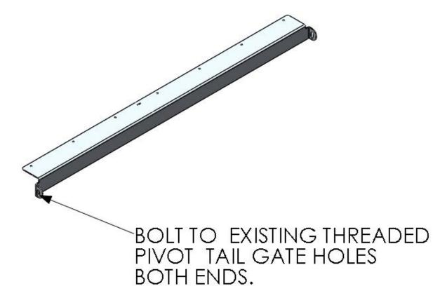
4. Mount filler panel assembly to load bin as shown.
