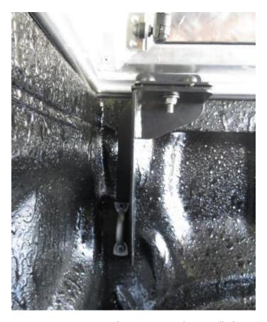
Figure 21: Front-Right Support Bracket Installed
