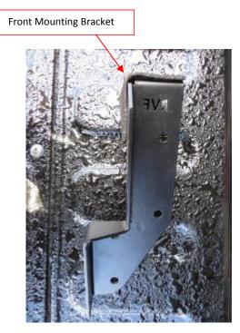
Figure 1: Front Support Canopy Brackets
