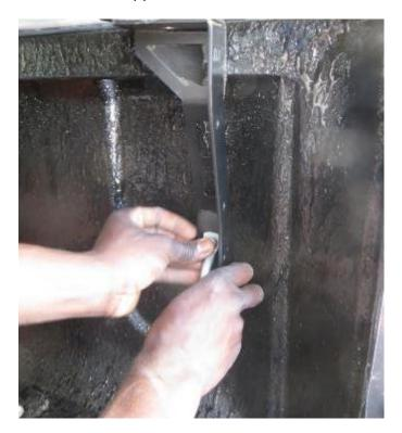
Figure 8: Aligning the Rear Support Bracket
