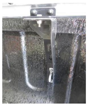
Figure 18: Rear-Right Support Bracket Installed
