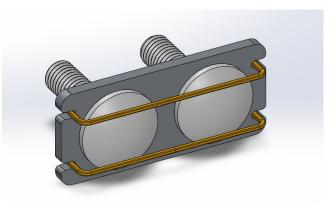
Assemble the nut plate, cup square and elastic band as shown in the image above. Slide this assembly into the rail in the load bin
