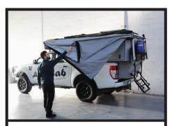
Step 4: Holding the strap, walk around to the front of your vehicle, to the front of the awning frame. Make sure that bystanders keep clear!
