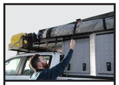
**Step 3**: Undo the three Velcro straps.
