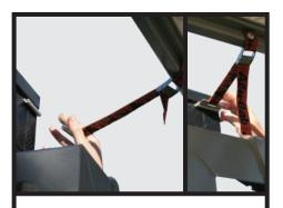
Step 4: Clip the strap onto the rail at the back of your vehicle.
