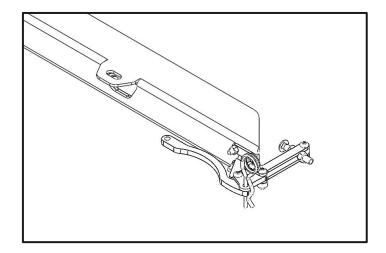
**Fig 2.** Table Slide Toggle Clamp
