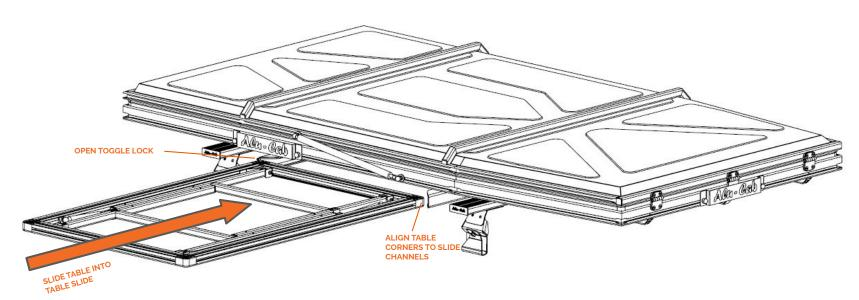
**Fig 6.** Alutable into Table Slide
