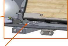
Slide M8x25 Bolts through and hand tighten
