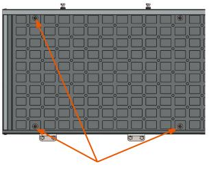
Slide in M6 Button Heads and oversized washer through holes
