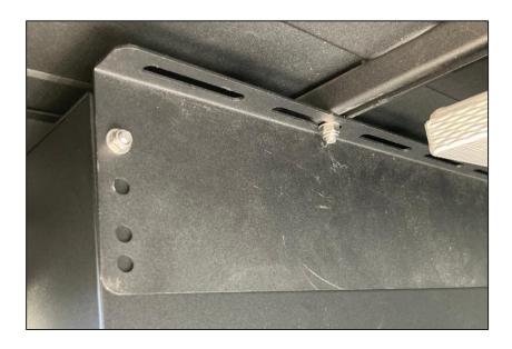
With the Top Bracket fitted you can adjust the bottom brackets. Ensure that they line up with slot cut outs on the canopy cupboard, and do not clash with the canopy mounting brackets.
