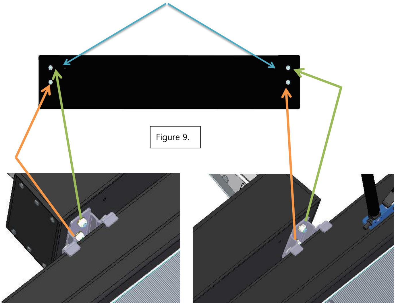
Place shower cubicle assembly with the bag on mounting brackets and secure shower cubicle to the mounting brackets using the same nuts that where removed in **figure 9**.
