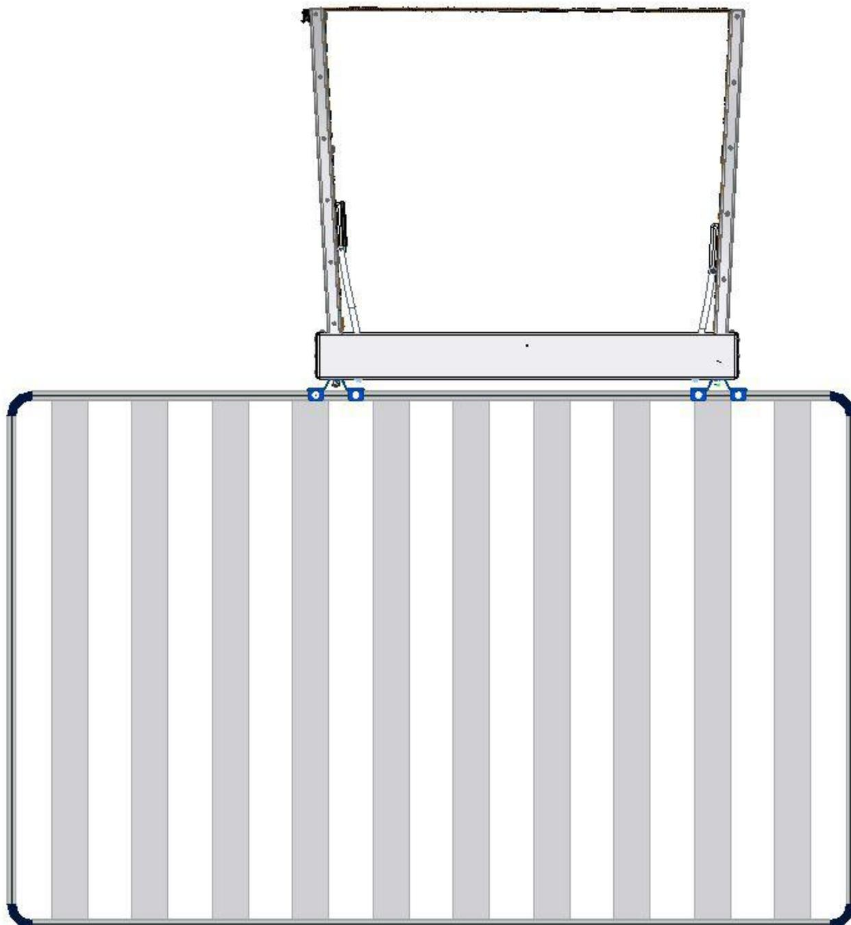
Position the Shower cube with brackets fitted, onto the Roof Rack to whichever position along the sides of the vehicle.
