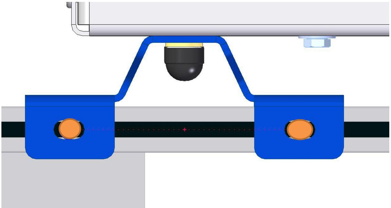
Use the slots on the brackets as a jig to drill 8.5mm holes to fit the M8x70mm bolts.
