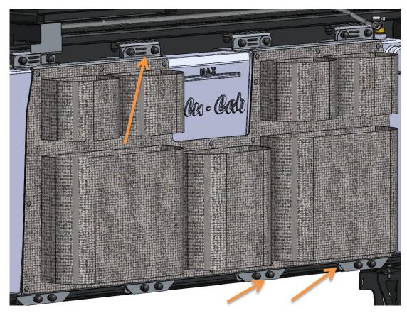
Place Plastic Nut Caps over all the exposed M8 Nuts and Screws
