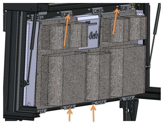
Fully tighten all Nyloc Nuts to secure the Water Tank in place
