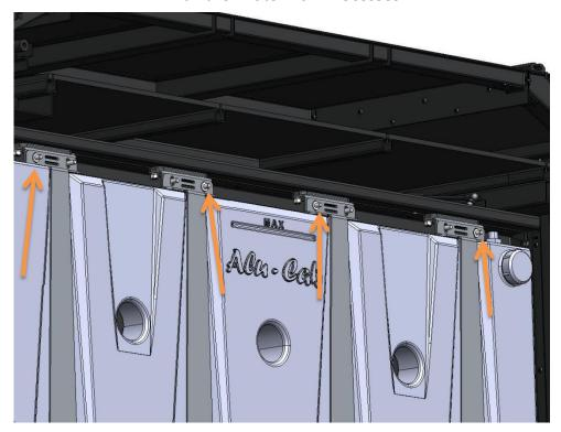
Place 4x M8 Flat Washers on the corresponding M8 Screws as shown
