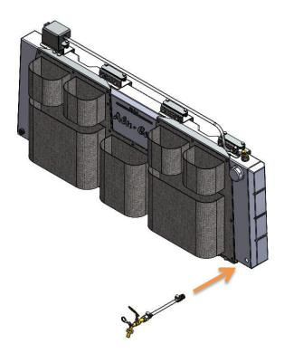
Add thread tape or thread sealant to the Male threaded hose fitting on the Tap Assembly and screw it into the desired Outlet on the Water Tank. Next, using your Drill, drill a 20mm hole in the desired location for your Tap, unscrew the Tap from its hose connector and screw it back through the drilled hole, sealing with thread tape or thread sealant. A 3m length of hose has been supplied to access most applicable locations for your tap mounting location.
