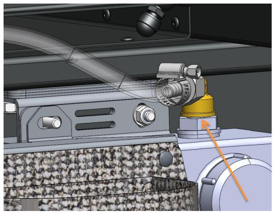
Place the Water Tank Breather assembly as shown, and screw on the connector to the Water Tank Bulk Head Fitting
