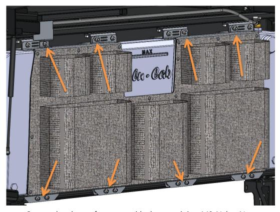
Secure the shown fasteners with the remaining M8 Nyloc Nuts
