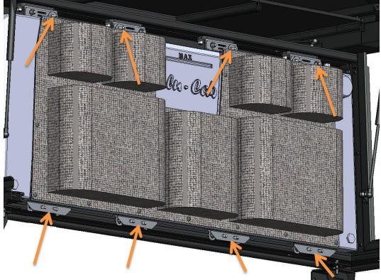
Place the Water Tank Cover Plate and Canvas Bag assembly over the corresponding Screw fasteners as shown
