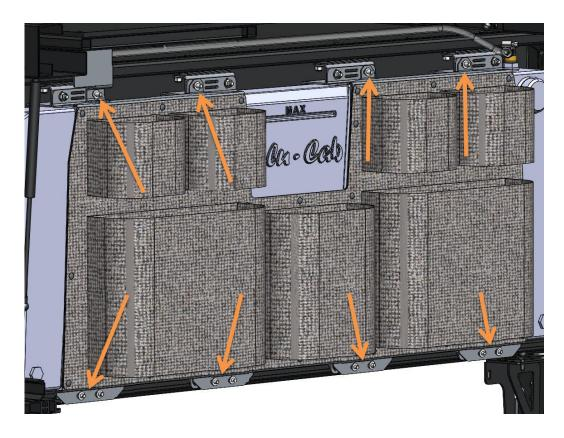
Place M8 Flat Washers over the shown Screw fasteners
