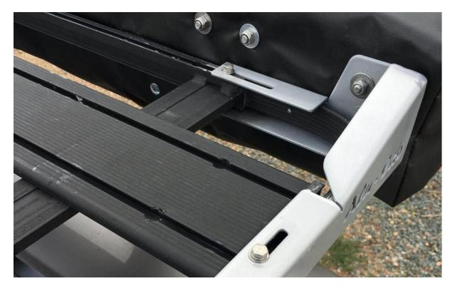
The K-9 brackets are universal and can be mounted either on the left or right side of the roof rack.
