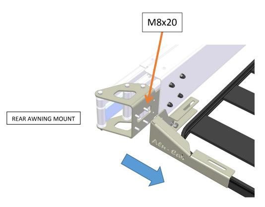
Line up the supplied brackets and and the awning to check that the awning's 270deg arm clears the vehicle.
