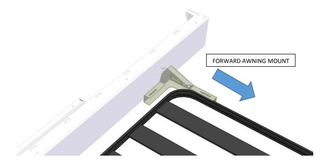
Test fit the front bracket supplied and mark the holes required to mount the awning. Drill through the awning with an 8mm drill bit
