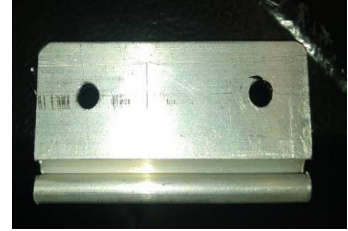
Figure 5: C-Clamp extrusion with holes drilled
