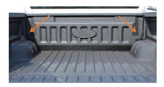
Mount the brackets on the LH and RH sides, making use of the four (4) factory mounting points either side, as indicated. Use the supplied M8X20 bolts, and M8 washers.
