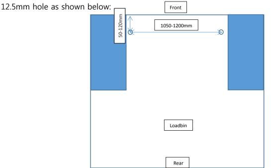
The measurements might vary depending on your load bin, but try to stay within the sizes indicated in the above diagram. Fasten the chain assembly as shown below:
