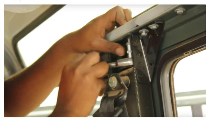
You will notice that there is no angle plate or aluminum for you to mount the door seals at the top of the door on the front 2 doors. These angles we supply separately. You will need to drill these into position, and apply bonding adhesive behind the plates.
