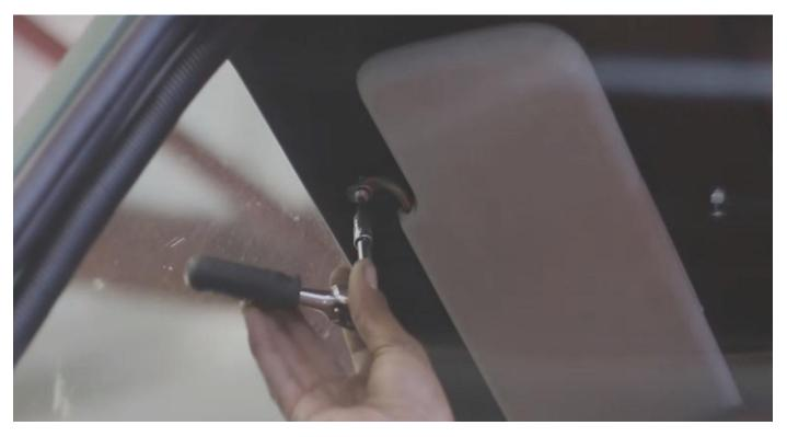
It is important to drill up at the front area where the sun visor will mount, using the existing holes from the sun visor. We recommend using a 7mm hole which will help to allow you to mount the roof console when fitting the final parts.
