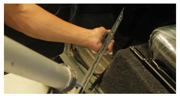
Once you have fitted the Icarus Roof Conversion, you can align the rubber door seal mount with the existing Land Rover's door seal mount area.
