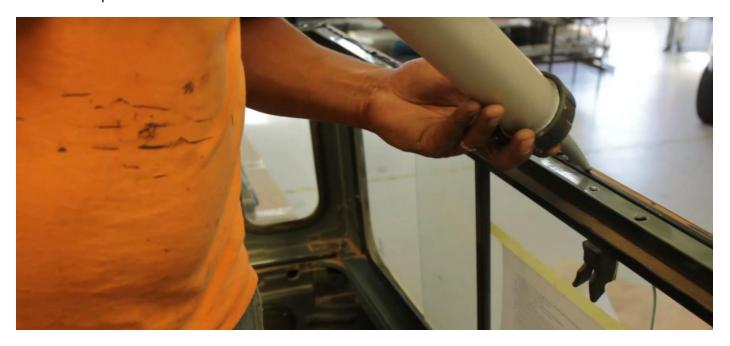
In the windscreen area, be sure to to apply at least 3 layers of bonding adhesive to help to prevent the chance of wind or water blowing through between the roof and windscreen area.
