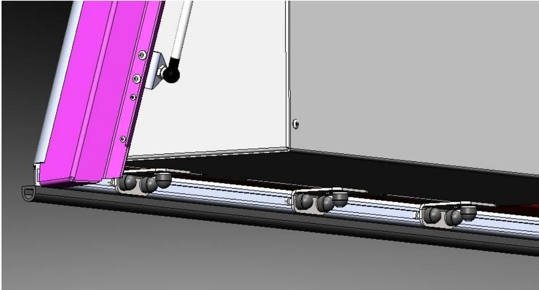
Bottom Brackets Assembled using M8 Hex Bolts into the nut Slot and M8 Cup square bolts into the canopy Cupboard. There are slots to adjust the position of the cupboard brackets to clear the canopy load bin brackets.
