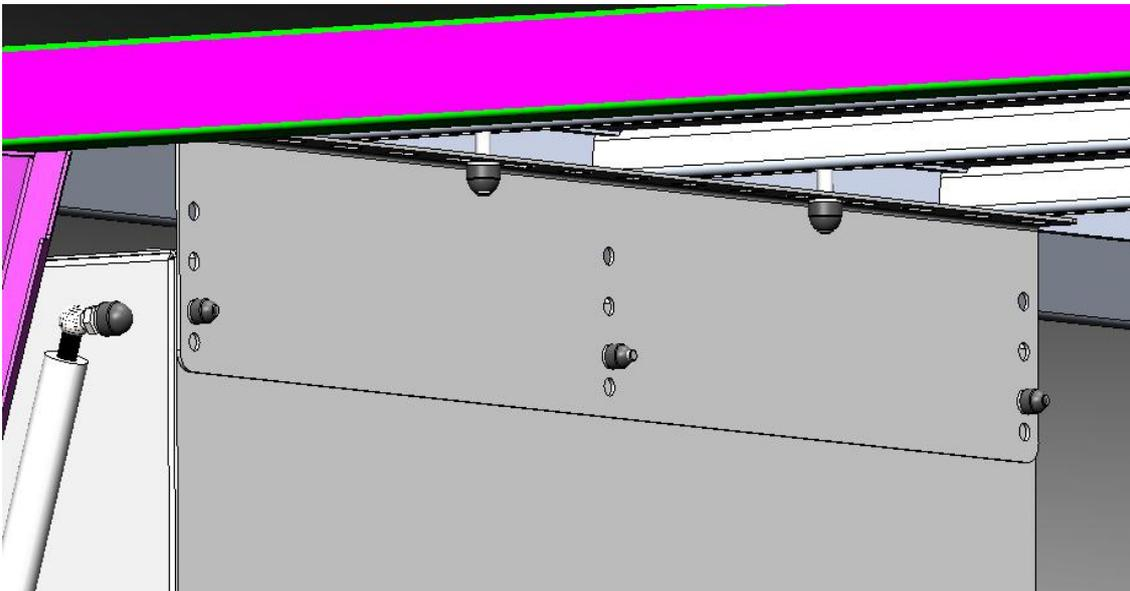
Top Bracket Assembled. Use M6x20 Button Head screws to bolt Bracket to the Cupboard and M8 Bolt Bracket to the Canopy Frame roof as shown. Bracket is height adjustable to suit multiple canopies. Remember to fit plastic nut caps over the nyloc nuts
