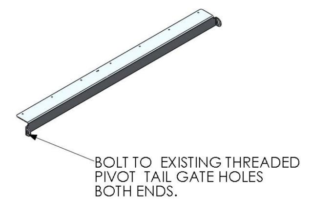
4. Mount filler panel assembly to load bin as shown.
