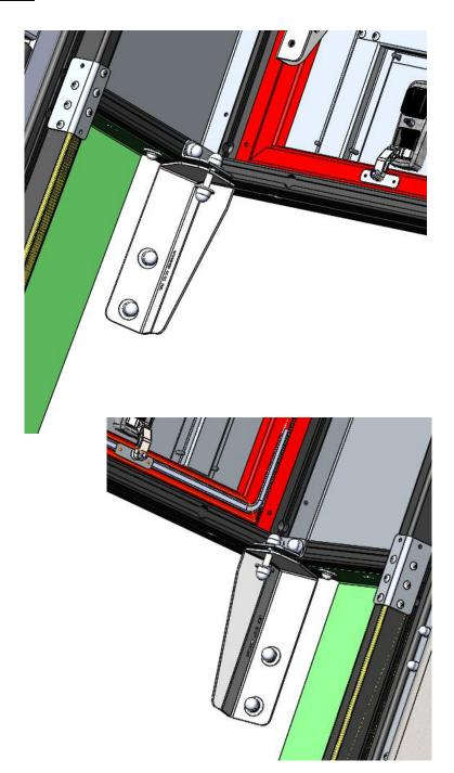
**NB!** The Canopy Camper must rest solely on the mounting brackets and no load is allowed on the load bin. Once this is completed, the Canopy Camper has been installed successfully.
