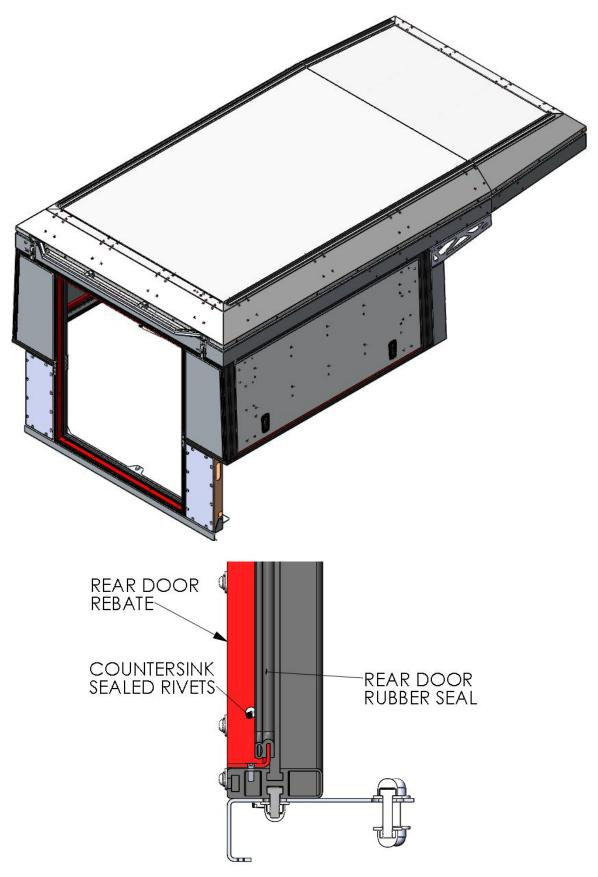
7. Fit rear door by mounting 4 x Butt hinges to camper frame as shown. Centre rear door, top to bottom and the hinge centers left to right. Also mount the door lock to the camper frame.
