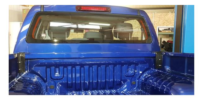
4. Images showing front mounting position of mounting brackets in load bin
