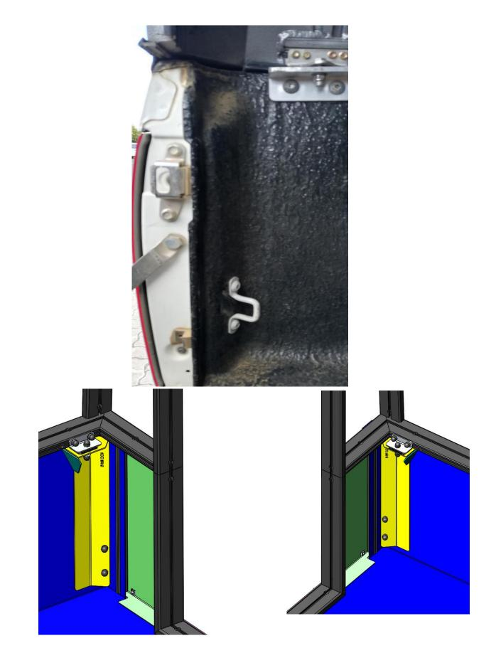
**NB!** The Canopy Camper must rest solely on the mounting brackets and no load is allowed on the load bin. Once this is completed, the Canopy Camper has been installed successfully.
