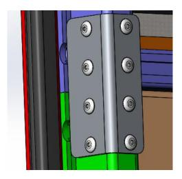
6.Fit rear door rebate with Ø4.8 x15 sealed countersink rivets as shown.
