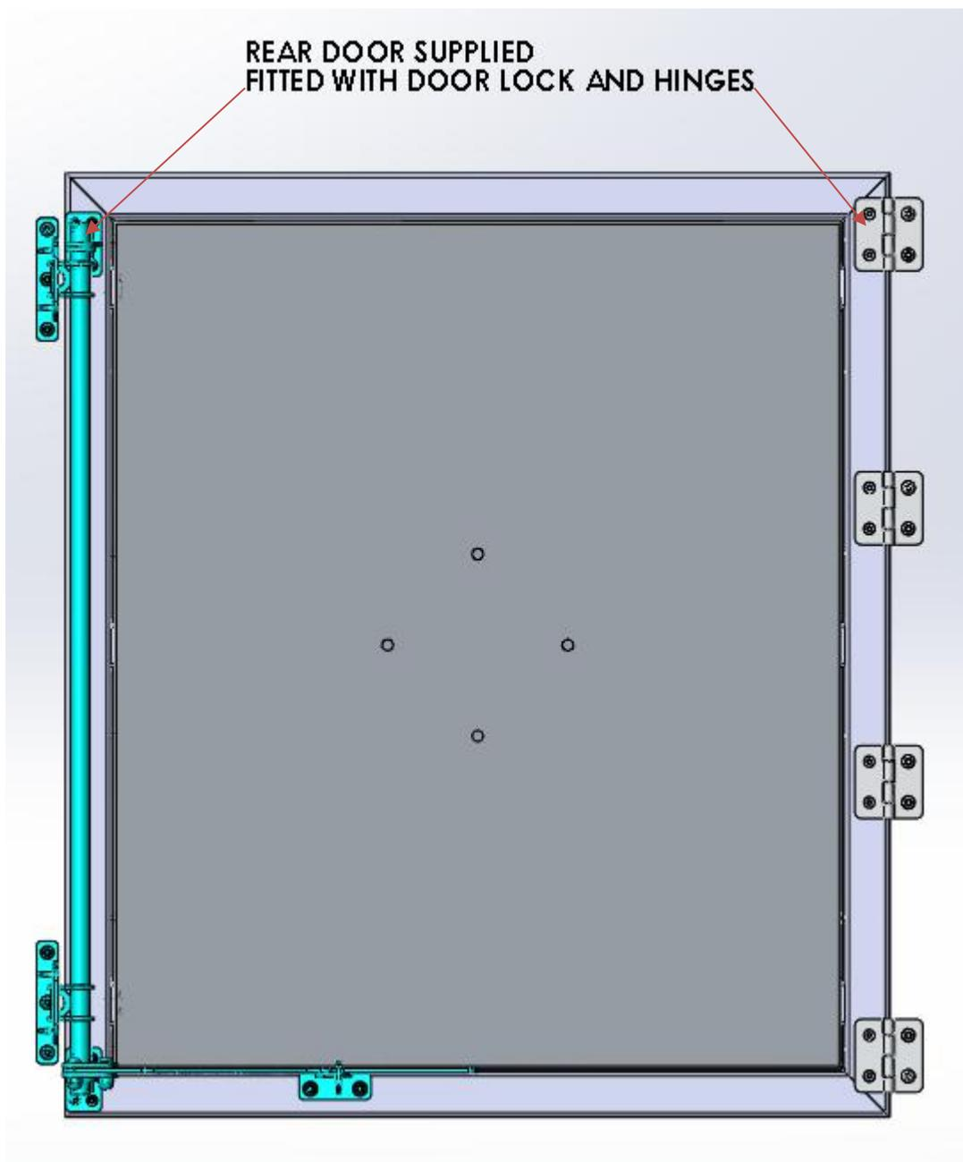
9. Attach hinges and lock to camper frame.
