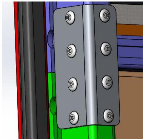
7. Fit rear door rebate with  $\text{Ø}4.8 \times 15$  sealed countersink rivets as shown.
