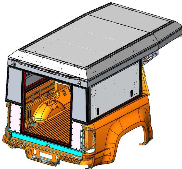
6. Connect rear filler panel assembly and base unit as shown.
