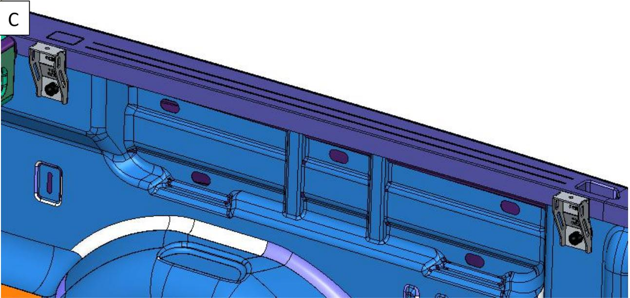
Add M8 nut caps, to finish off the bracket installation. You will now have four brackets installed at the front and rear, on both the LHS and RHS. You can now continue with the rest of the fitment.
