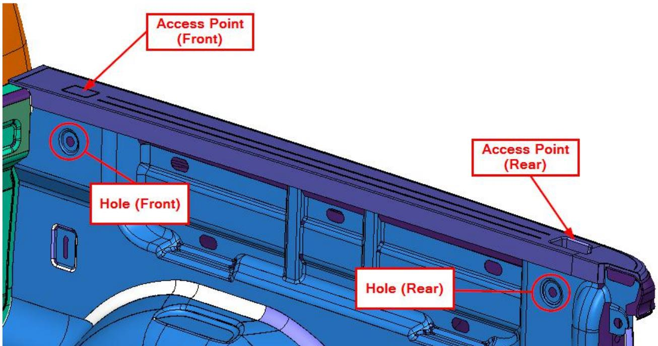
The front and rear mounting brackets must be installed at this stage, as there will be no access to the fasteners once the Canopy Camper is seated on the load bin.
