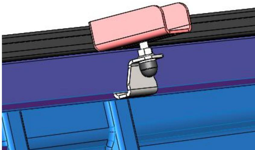
**NB!** The Canopy Camper must rest solely on the mounting brackets and no load is allowed on the load bin. Once this is completed, the Canopy Camper has been installed successfully.
