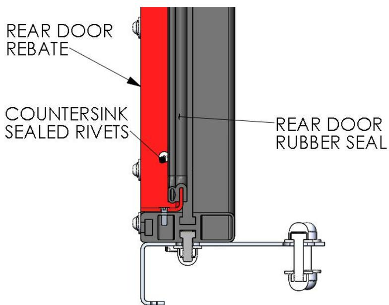
8. Fit rear door by mounting 4 x Butt hinges to camper frame as shown. Centre rear door, top to bottom and the hinge centres left to right. Also mount the door lock to the camper frame.
