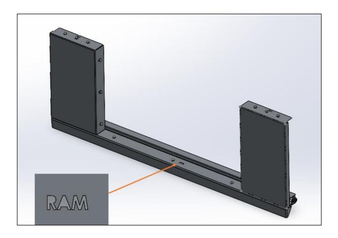
The Rear Filler Assembly is made up of three main sheet metal parts, the inside boxes as well as the bottom filler brac.
