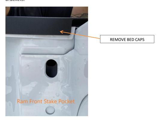
With the bed cap removed it is possible to access the stake pocket.
