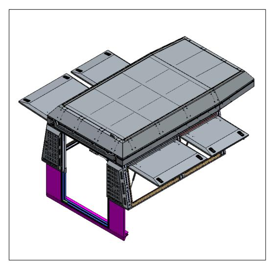
Attach the gasket material to the lower seating surface of the Canopy Camper's base frame - Refer to the stand alone Fitment Instruction for this process.
